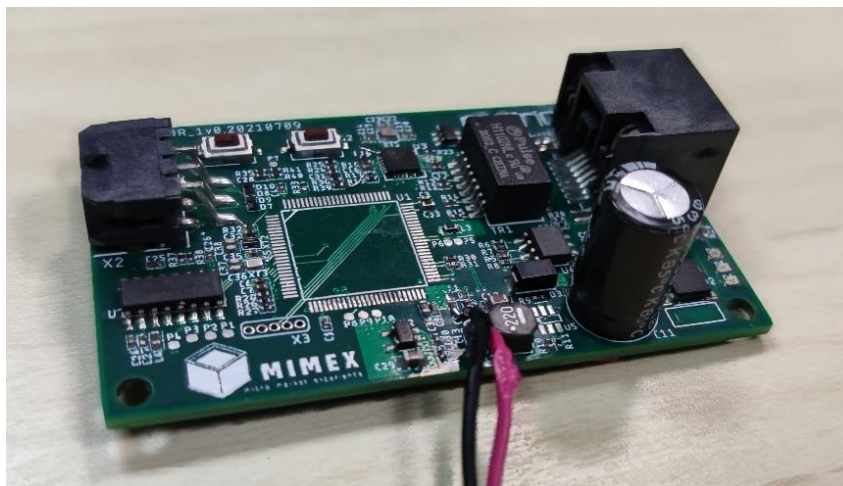
Figure 13 – PCB prepared to work with an external power supply.
