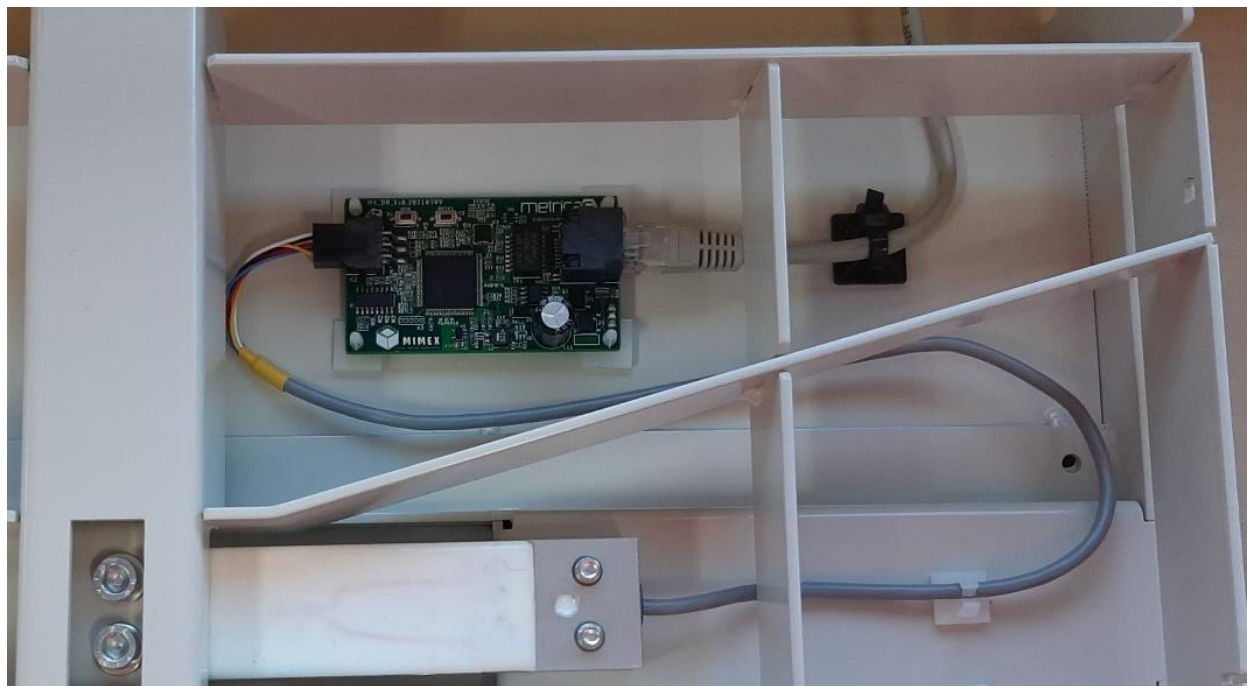
Figure 8 – Digital Reader inside the weighing system
