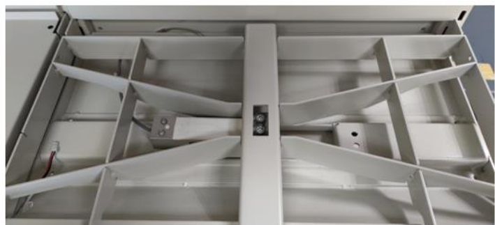
Figure 7 – SPO 40 Load Cell and Location
